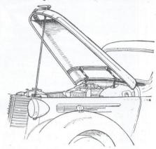
The top of the bonnet lifts for access to the engine, a rod holding it in place; bonnet sides can be detached if required.
