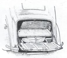
The spare wheel is mounted below the luggage boot and secured with a strap, and the lid of the boot serves to accommodate extra luggage.
