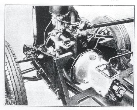
The compact Eight engine is mounted well forward on rubber. An extra deep boxsection of the frame is employed at the front to give rigidity.
