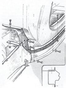
How the body sills are bolted to the flanges of the frame channel sidemembers to form a box-section when in position. The dotted lines show which bolt holes on the body correspond to those on the chassis.
