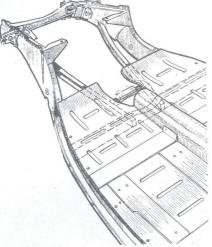
Frame details at the front of the new Eight, showing the platform floor.
