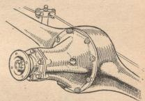
The rear axle casing is made of two pressings welded together on the centre line. (Left) The brakes are of the full Girling pattern with 8-in. cast iron drums.
