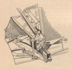
The steering employs the usual Austin hour-glass worm and sector, and is anchored at the front extremity of the frame. Many Interesting Features in a Model Available with Open and Closed Bodies to Replace the Seven and Big Seven
