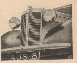
MODERNISTIC. A pleasing new front arrangement is a feature of the Austin Eight, in which the grille is built up of ten die-cast segments
