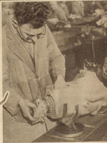
GEARS. A special section is devoted to gearbox production and these, like the engine, are thoroughly tested before being passed as ready for fitting to the car.
