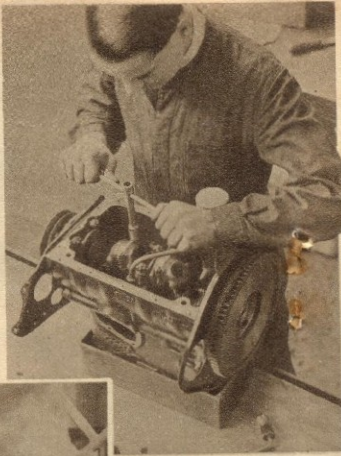
ASSEMBLY BENCH. An Austin Eight engine has its big-end bearings finally tightened down before the sump is put on.
