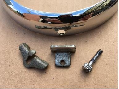
Some head light rims were of a type with a bottom hole, which needed different mounting materials like the catching bracket as shown in the image above.
