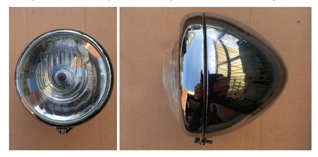
A8R Reflector kit with new reflector and re-use of original glass with H4 12V or 6V Halogen
