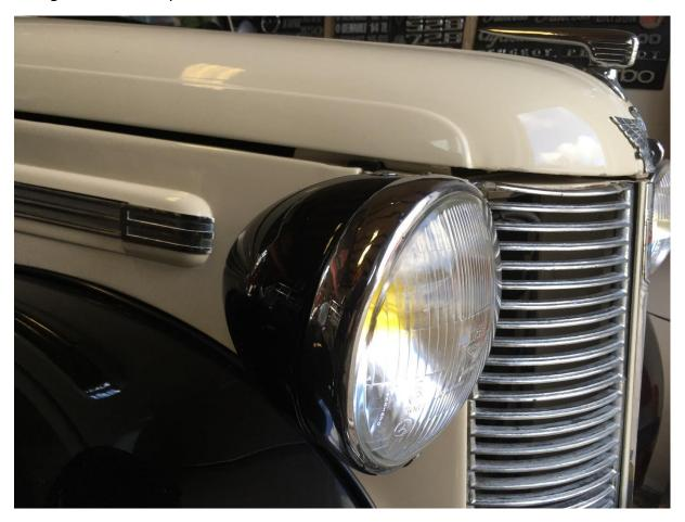
Example of a Lucas L133 pre-war head light with Lucas 700 conversion kit. The rim on the head light converts from 6 % to 7" Which make most Lucas 700 head light insert kits suitable to fit.
