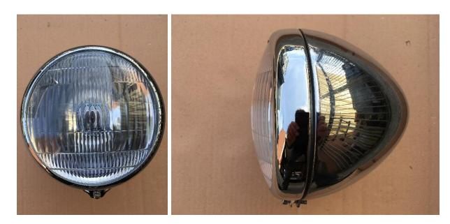
A8R Reflector kit with loose reflectors and loose glasses with H4 12V or 6V Halogen
