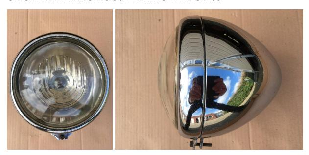
Original head lights 6  $\frac{1}{2}$  inch with internal magnetic high beam still installed.
