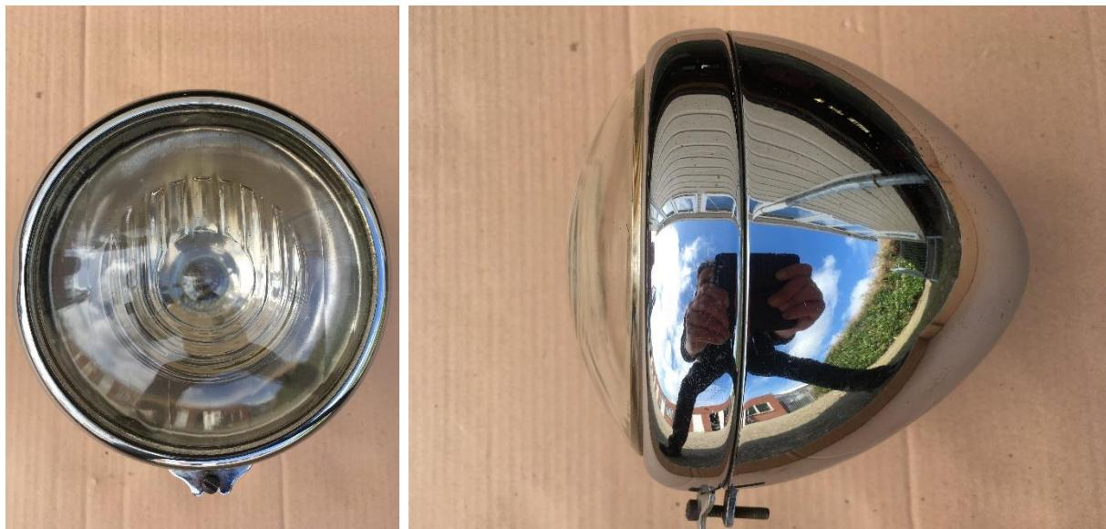
*Original head lights 6 ½ inch with internal magnetic high beam still installed.*
